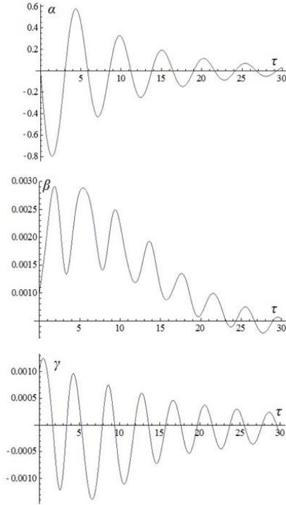
**Figure 5. The transition decay processes for  $\theta_A=1$ ,  $\theta_C=0.5$ ,  $k=0.2$**
