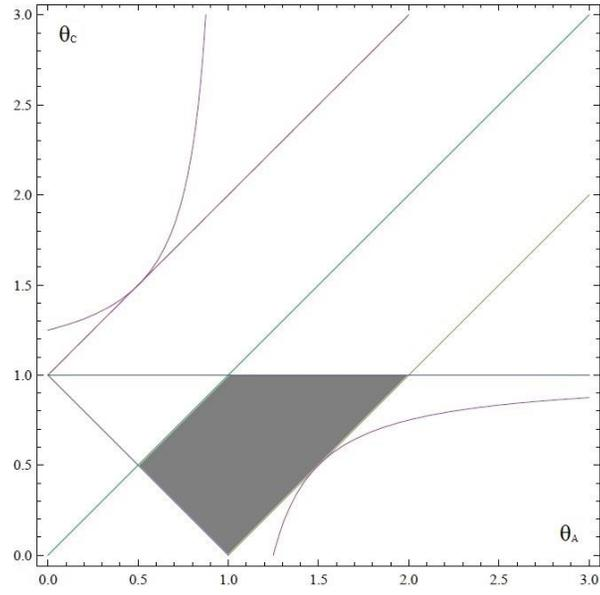
**Figure 3.** The domain of the conditions of asymptotic stability (grey) for  $k=1.0$ .
