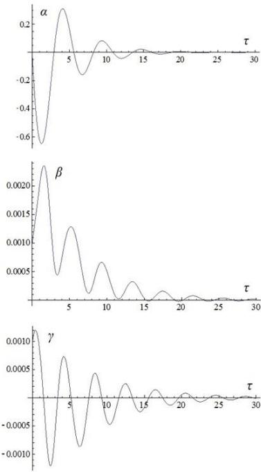
**Figure 6.** The transition decay processes for  $\theta_A=1$ ,  $\theta_C=0.5$ ,  $k=0.5$
