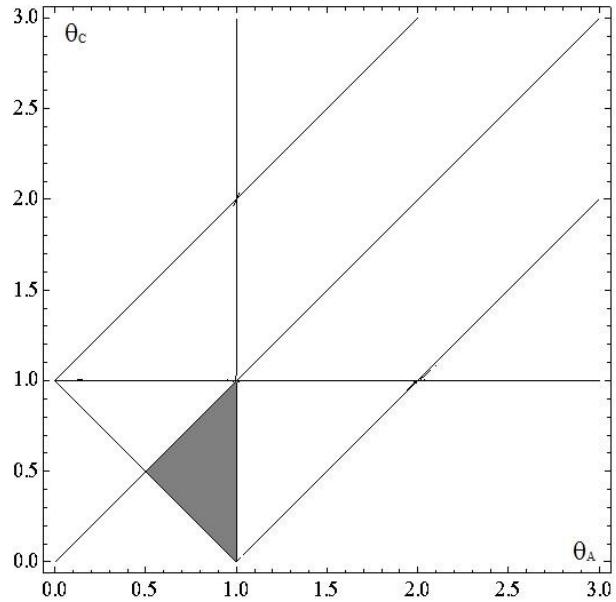
**Figure 1.** The domain of the conditions of asymptotic stability (grey) for  $k=0.01$ .
